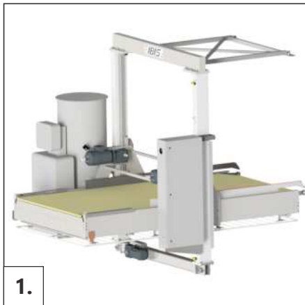
Automatic loading and unloading system Atlas with vacuum cleaner (option)
