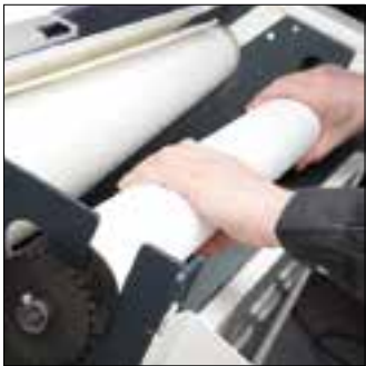
Moulding belts Ultra-fast change of belts without dismantling the machine
