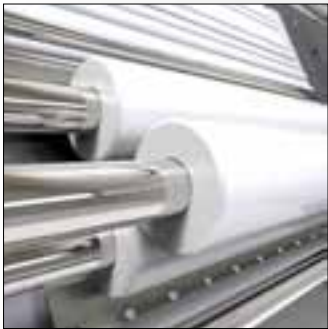
Three sheeting rolls made of food grade polyethylene. The first roll directs the dough towards the other two rollers. This succession of rollers allows for progressive rolling of the dough.
