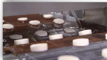
Enrobage partiel Partial coating
