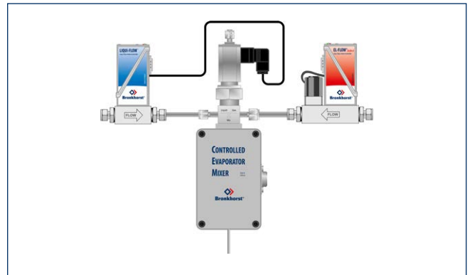
Single carrier gas supply, no dilution, thermal liquid flow meter.
