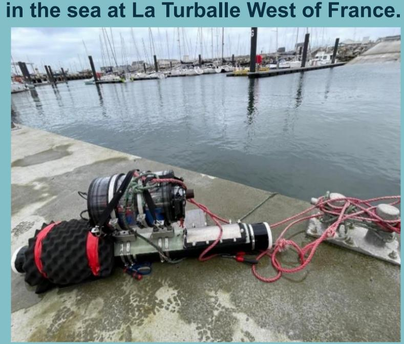
Foam insulation (to simulate mussels growth) on submarine
