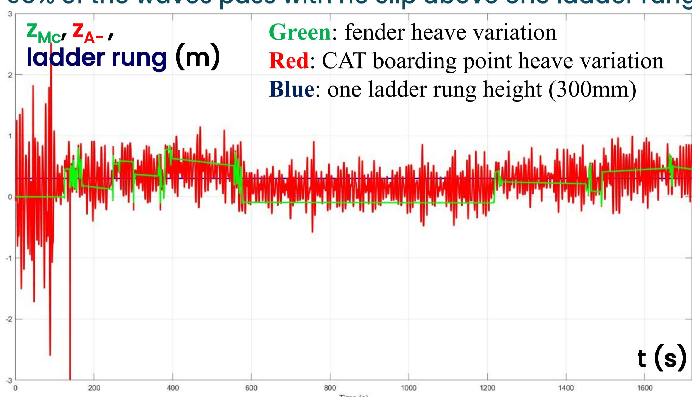
For a 2m significant wave height & 7,5s peak period , less than 95% of the waves pass with no slip above one ladder rung
