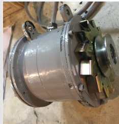
SHUTDOWN VALVE MECHANICAL- OVERSPEED VALVE
