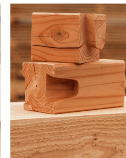
Column cap dovetail joint
