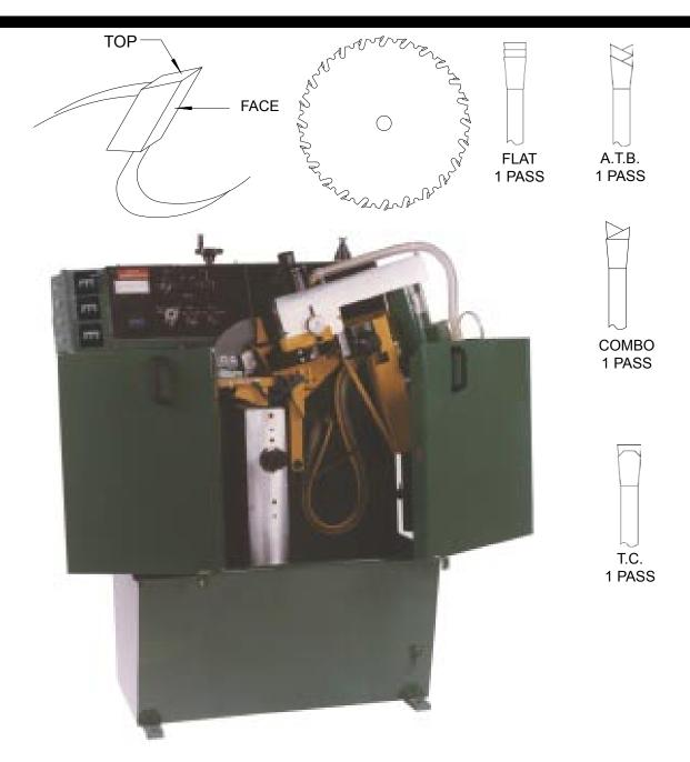
The Wright W-150 HD E model sharpens the top or face of circular saws. Heavy duty construction increases grind accuracy, productivity and machine life.
