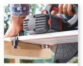
The fixed and adjustable stops on the underside of the rail allow the system to be used for angle cuts from +60° to -60°.
