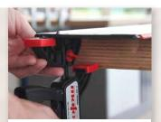
With 2 fixing clamps the guide rail can be fixed additionally on the workpiece.
