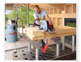
Whether you're cutting longways, crossways or at an angle, the plug-in supporting system for pressure-resistant and flexible insulating materials can be configured to suit any situation.
