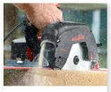
The chip management system was designed and optimized for cutting fiberboard. The superb chip removal system offers substantial benefits, including when executing plunge cuts in the fiber direction.
