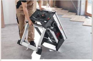
Assembling and disassembling the ERIKA are simple one-man jobs. You can unfold the built-in fold-away ssupport within seconds and without tools. - The /Quickstand\.
