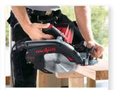
By retracting blade alongside the second handle, offering up the machine is easy and safe, especially when executing bevel cuts.
