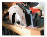
A handy machine combined with a guide rail ensure high precision, as shown when cutting doors to length.
