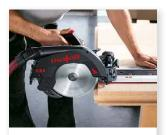
Thanks to the unique tilting system, the sawblade always cuts directly along the rubber lip, irrespective of the angle setting.
