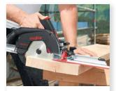
One-stop solution: in view of the saw's connection to the guide track, this is the world's first and only single-handed cross-cutting system.
