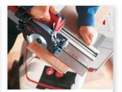
Fastening the portable circular saw to the KSS rail creates a very practical single-handed cross-cutting system.
