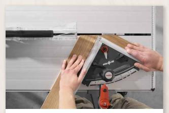
The multi-purpose guide fence allows two miter cuts without changing...
