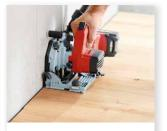
Perfect edging: the circular saw's spacers enable you easily to make exact expansion joint cuts with widths from 13 mm (1/2 in.).
