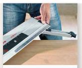
Place the assembled unit, comprising the angle fence and guide rail, on the workpiece.
