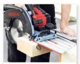
An ideal application for guide L is cutting structural timber to length, with a max. cutting depth of 82 mm and a max. cross-cutting length of 370 mm.
