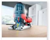
Innovative CUmax sawblade clamping ensures a positive fit because of a wedge pushing against the blade. This design reliably fastens the sawblade so that it cannot be displaced.
