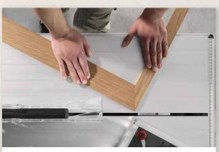
$\dots$  or adjusting the fence. The result: perfect  $90^{\circ}$  joints.
