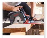
One-stop solution: with the cross-cutting system, the machine is permanently attached to the guide track.
