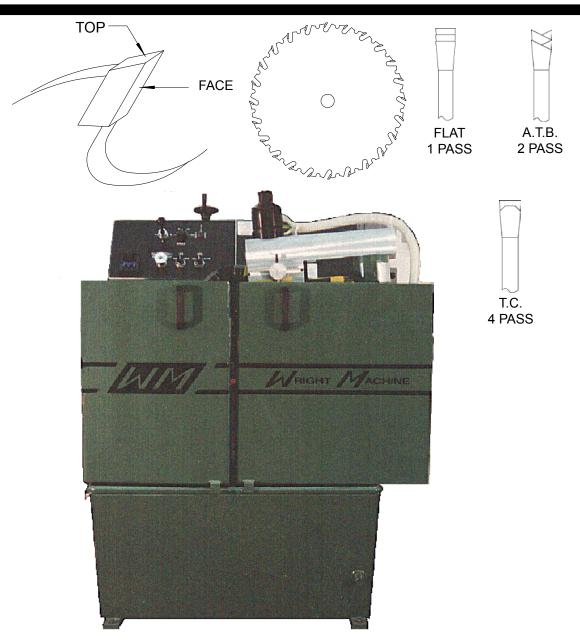
The Wright W-150 HD Sharpens the top or face of circular saws. Heavy duty construction increases accuracy, productivity, and machine life. With such easy operation and maintenance you can count on the W-150 HD A's performance year after year.
