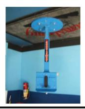
This "NEW" Powered Post bracket will raise and lower with the Air Back Feed and an additional bracket if needed, dependant on saw size.
