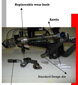
Clamp Screws & replaceable threaded bushing
