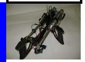
Repetitive motion injuries are costly to a sawmill but also painful for the Filer, The Magnum Swage was created to reduce the effort and reduce repetitive motion concerns on swaging and also produce a proper swage for improved saw performance.
