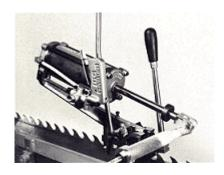
Armstrong offers a selection of air swages built especially for sash gang saws. Popular models of band, circular and sash gang swages are available in both hand and air versions.
