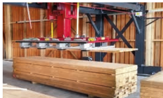
Gantry robot 500 t on mobile framework Maximum capacity 500kg up to 7 cycles per minute
