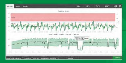
Sound level measurement curve SPL (top): At 16:35:59 the SPL exceeds the set limit (red area), the feed (blue line) is immediately slowed down briefly. This effectively prevents damage to the saw blades.
