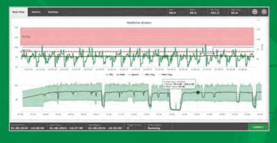
Sound level measurement curve SPL (top): At 16:35:59 the SPL exceeds the set limit (red area), the feed (blue line) is immediately slowed down briefly. This effectively prevents damage to the saw blades.
