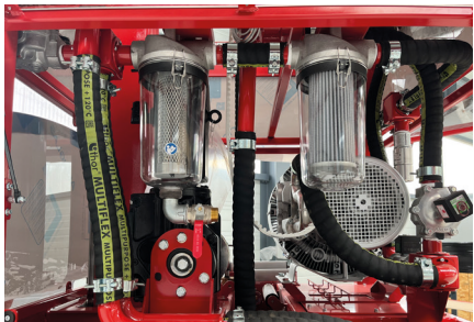
Filtering system for wet and dusty environments
