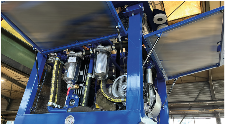
4 doors with springs for easy maintenance
