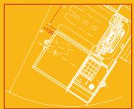
The reach capability (X-dimension) has been improved to 150mm, without changes to the truck dimensions. The added outreach provides operational benefits, with improved flexibility for loading and unloading, and use of a 1,200mm deck in circumstances that would otherwise require 1,400mm – improving storage capability.
