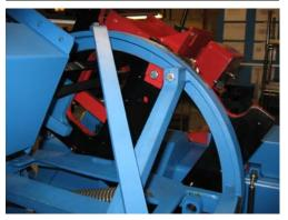
Remove existing rocker assembly and carriage and replace with new upgrade kit, bolt on existing belt tensioner and install guards.
