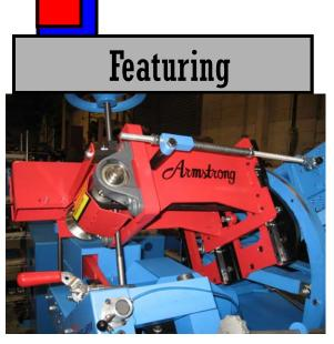
This "NEW" upgrade kit comes complete with the items needed to replace head rocker points, rocker cone screws, guards, mounting hardware and linkage on #4 sharpener or VariSharp.
