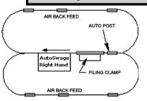
The Armstrong AutoSwage is available as either a right or left hand machine. Saws of the same hand as the AutoSwage encircle the AutoSwage. Saws of the opposite hand as the AutoSwage are looped in front of the machine. As shown in the illustration, one AutoSwage can swage & shape both right and left hand (or double cut) band saws by using two sets of post brackets and two air back feed units
