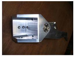
Remove existing feed arm cone screws and bushings ~ mount in place of Old feed arm 2 bolt installation virtually can be installed in minutes.
