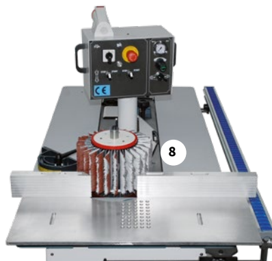
8 Spazzole a settori intercambiabili MultiBrush Multibrush - brush with interchangeable segments
