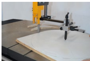
Tagliatondi - Levigatore Circular cutting and sanding device
