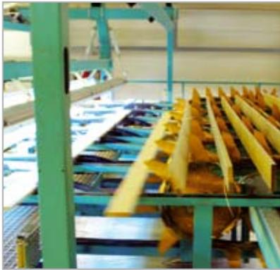
Automatic scanner grading, in between the pieces are turned.
