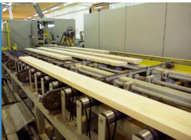
SMB's compact line is used especially in jointing larger dimensions for log-house manufacturing purposes.
