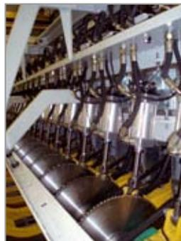
Cutting the green timber very accurately to the selling length allows to increase the green wood chips and thus to improve the productivity. One of the efficient cutting methods is trimmer sawing shown in the picture. For extremely high speeds we recommend the Jartek Free Cut system.
