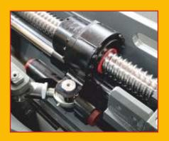
The unique award-winning Baumann VRS outreach system provides smooth and accurate mast travel. A bespoke valve block allowed us to double the Archimedes spindle thread size and corresponding number of bearings, halving of the pressure required between them, providing greater control and the ability to seal the spindle head.
