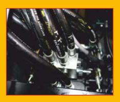
The EGX utilises a bespoke steering axle and flow matching hydraulic system. Through closed-loop control, the hydraulic pressure is adjusted depending on the load, saving energy and improving efficiency.
