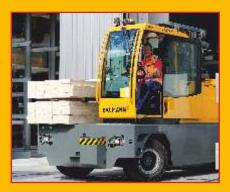
The EGX has two drive motors and larger capacity and longer run time 120v battery, offering the best running hours in its class. Add the panoramic cabin, load sensing, joystick control, full road-legal LED lighting and precise mast control and the offers true engine-like performance.
