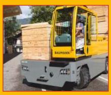
Once the platform is fixed in the horizontal position, the load remains stable even on uneven ground. Cornering speed is automatically reduced if safe truck parameters are exceeded and the incredible optional SafeLoad Assistance warns operators if potentially dangerous overloading situations occur.
