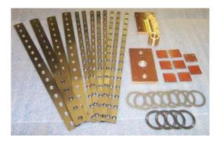
Super Duty Armstrong band saw stretcher rolls include these hardened steel liners, thrust bearings, brass bearing blocks, micarta shoes and brass insert for the pressure screw. Super Duty machines allow the operator to bring more pressure to bear on the saw for faster tensioning without dishing. Standard duty stretcher rolls can be upgraded and rebuilt to Super Duty configuration only at the Armstrong factory.
