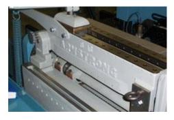
Close-up shows the steel slides installed in the ways of a 20-year-old stretcher roll. Note also the replaceable micarta "shoes" that slide against the hardened steel liners of the Super Duty stretcher roll. These "tighter" Super Duty stretcher roll machines work faster and require less maintenance.
