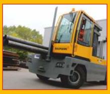
Once the platform is fixed in the horizontal position, the load remains stable even on uneven ground. The compact footprint, great visibility and tight turning circle allow complete confidence in operator safety and load security.
