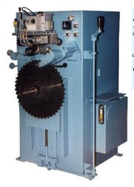
One AUTOTIP can be equipped to tip both band and circular saws. For example, a single AUTOTIP machine can tip all the saws in a sawmill with seven band mills and 60 circular saws. It takes just five minutes to change this machine from tipping circular saws to tipping band saws.
