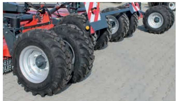
Various wheels and tyres configurations, including option tandem pendulum axles.
