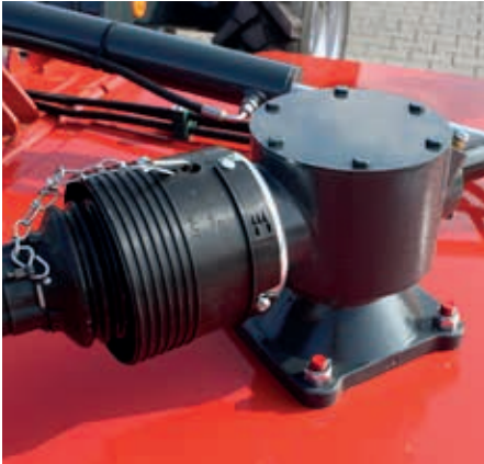
Spindle gearbox - with breather 180 hp rating - oil capacity: 3,5 liters
