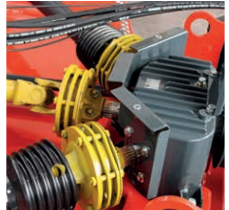
Secondary shafts with 2-disc slip clutch each.
