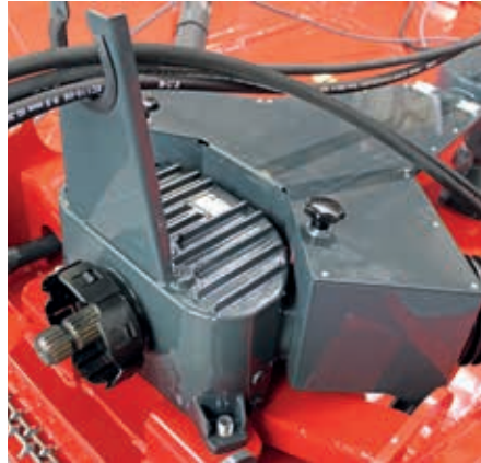
Splitter gearbox - with breather 290 hp rating - oil capacity: 3,8 liters
