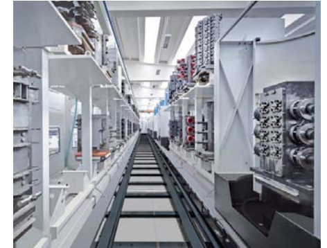
Eight horizontal work station: production of transmission boxes and gears
