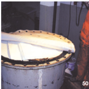
49 - The CARPI perimeter seal has been tested and approved by ISMES in a full scale test performed in a pressure vessel, applying water heads up to 25 bar.
