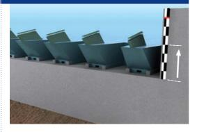
Installing Fusegates on the spillway sill increases the normal reservoir level while maintaining the dam's safety level.
