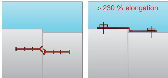
CARPI external waterstops can resist larger movements than traditional embedded waterstops. Their placement does not interfere with construction of the dam.
