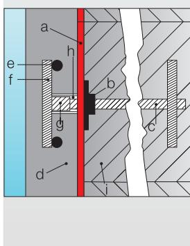
Detail of precast panel anchoring
