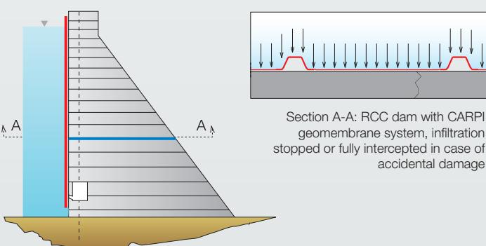
Cross-section: the formation of cracks after construction does not affect the CARPI system
