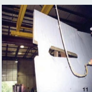
11 - Testing tensile strength of geomembrane strip between panels.
