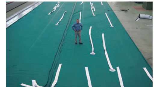
▲ Up to five rolls of geomembrane material can be seamed together to make a mattress roll of up to 10 m wide and custom-made length.
