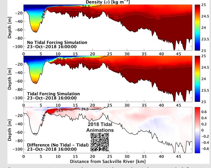
**Above** Density snapshots with and without tidal forcing (middle and top respectively), and the difference between the two simulations (bottom).
