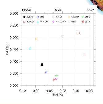
Through the analysis of bias and the RMSE distribution diagram between SST fusion products and Argo in-situ data, the RMSE ranges are from 0.3233 (OSTIA) to 0.5180 (MGDSST). The RMSE between NMEFC fusion products and Argo in-situ data is 0.3861, which is at the middle level of comparative analysis of SST products, ranking fifth out of 10 fusion products.
