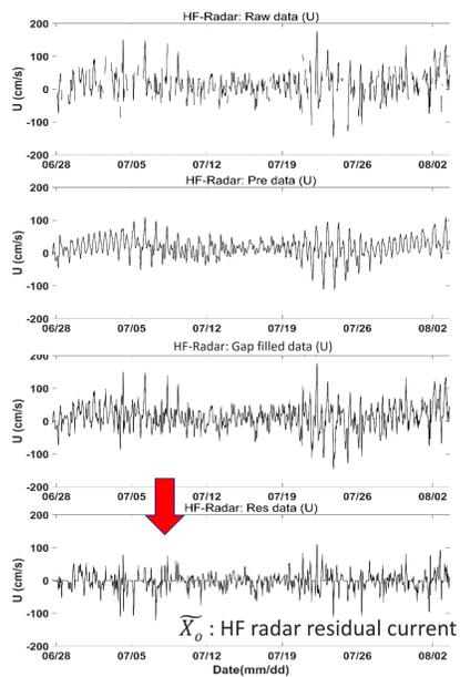
Fig. 3. The process of obtaining HF radar residual currents by performing harmonic analysis on raw HF radar data to fill gaps and applying harmonic analysis three times. The residual current from HF radar is then combined with the tidal current from the numerical model to be used in data assimilation
