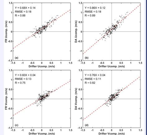
Fig. 5. Comparison with surface currents from drifters. Root mean square error (RMSE) and correlation coefficient (R) were used for assessment
