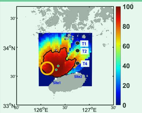
Fig. 2. Distribution of HF radar total vector data coverage (%) for July 2020 at Sites 1 and 2. The black contour line represents the 80% data coverage threshold. Green circles indicate the locations of ocean buoy observations, blue circles denote ADCP observation sites, and the orange circle marks the positions of seven drifter observations
