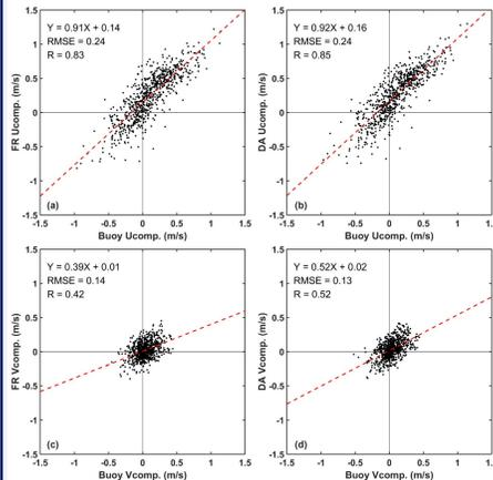
Fig. 4. Comparison of model surface currents with observations from ocean buoys for both u- and v-components in FR (a, c) and DA (b, d)
