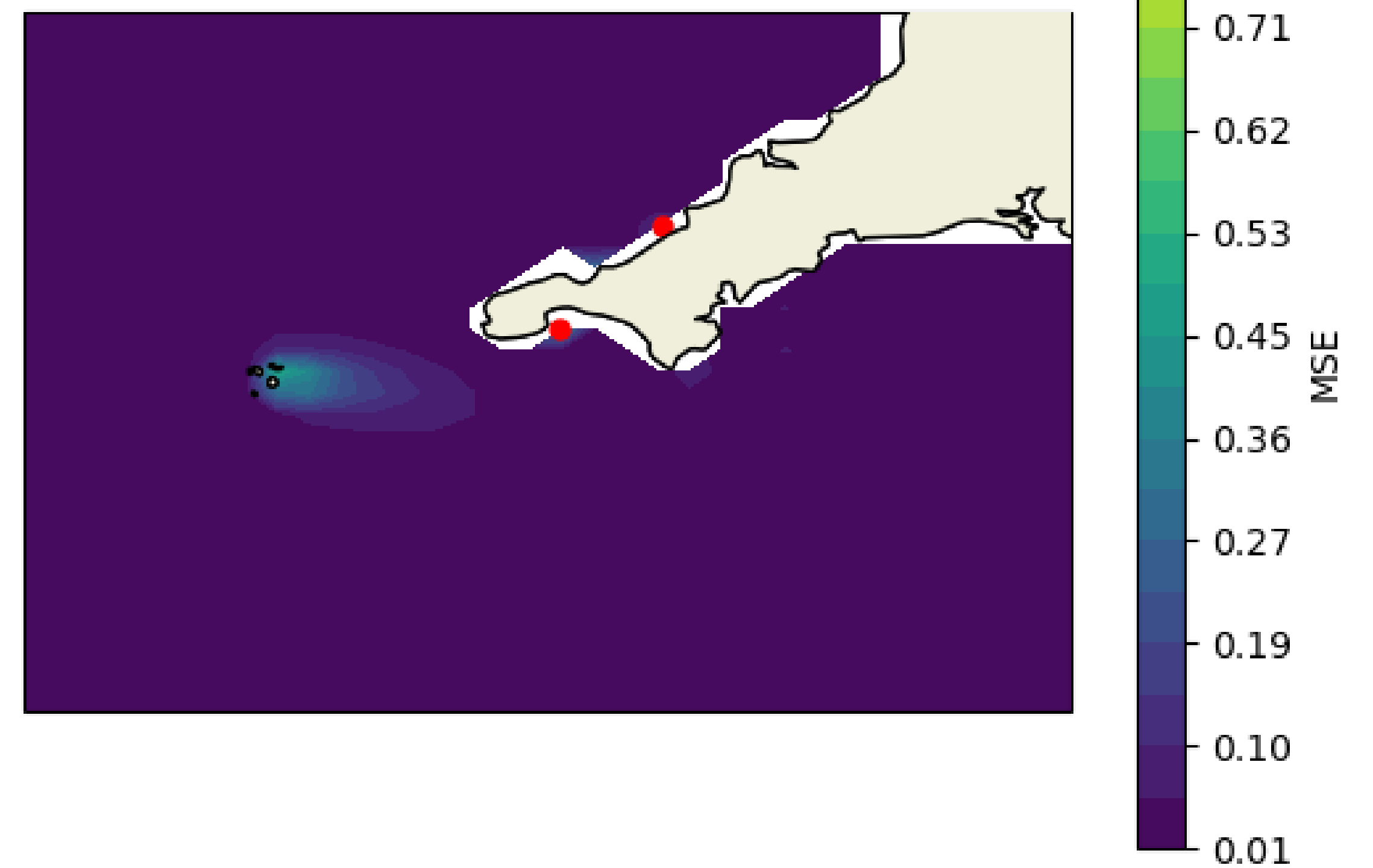
Mean Squared Error Significant Wave Height (Hs) 2022 MaLCOM bias corrected MO forecast vs HC
