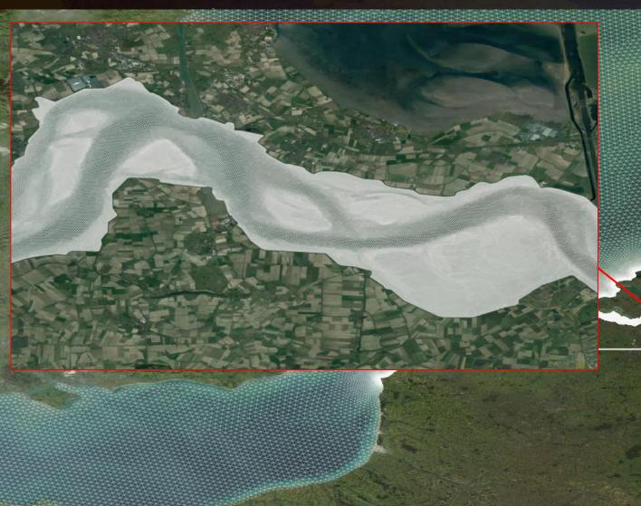
**SLIM2D**: depth-averaged barotropic Wetting and drying algorithm (tidal flats
