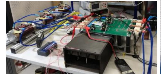
Industrial Realization of a 1,7 kV / 100A Full-SiC CSI Module
