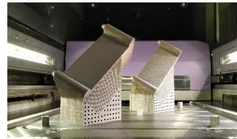
Methanation reactor and complex internal structure
