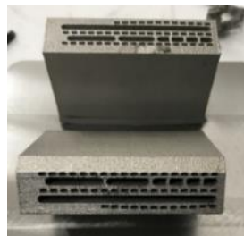
Thin channels and walls (Source: CEA Tech/LITEN)
