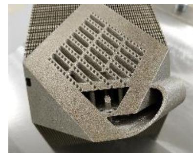
Methanation reactor and complex internal structure
