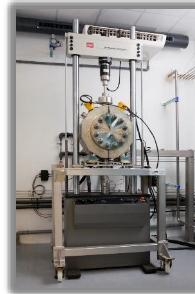
Mechanical testing up to 40 MPa bar H 2
