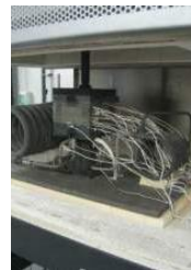
Electrochemical test rig (large stacks 6 kW) Pressurized test rig (30 bar) upon construction
