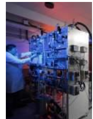
Electro-chemical test rig (SRU and small stacks 3 kW)
