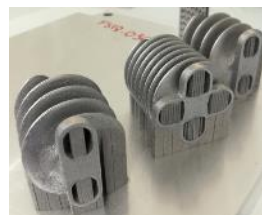
Complex absorption exchanger reactor
