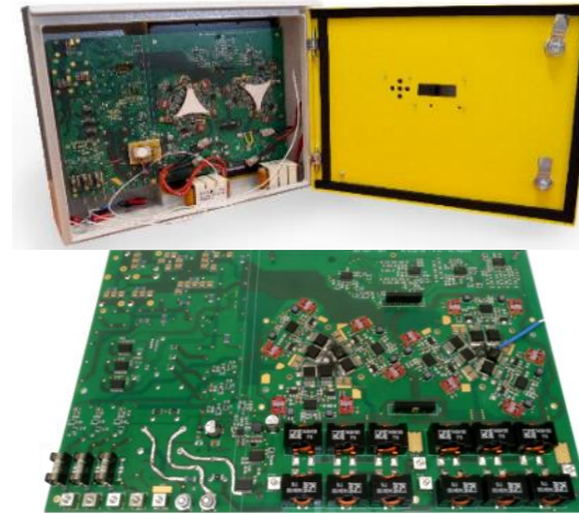
Industrial Realization of a 1,7 kV / 100A Full-SiC CSI Module
