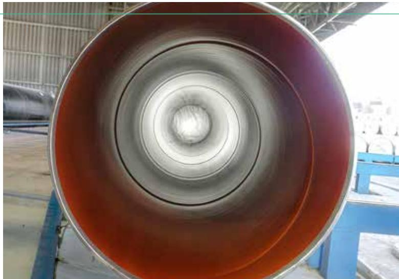
Tosçelik manufactures spiral welded steel pipes in compliance with API, ISO, EN and DIN standards.
