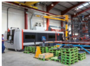
2 laser cutting machines for steel sheets
