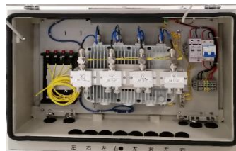
Integrated chassis for trackside AP Compliance with trackside shockproof specifications; IP66-rated protection
