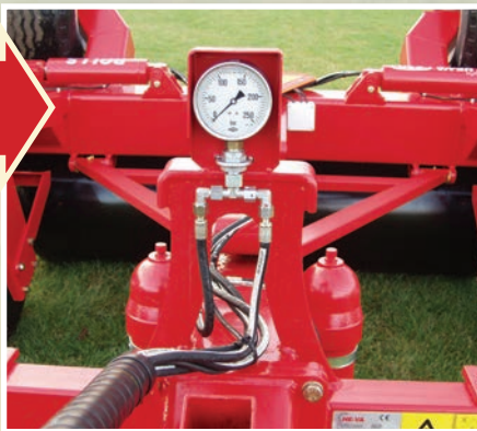
2 Even with a basic sprung weight transfer system the hinges at the centre roller section negate much of the transfer effect.
