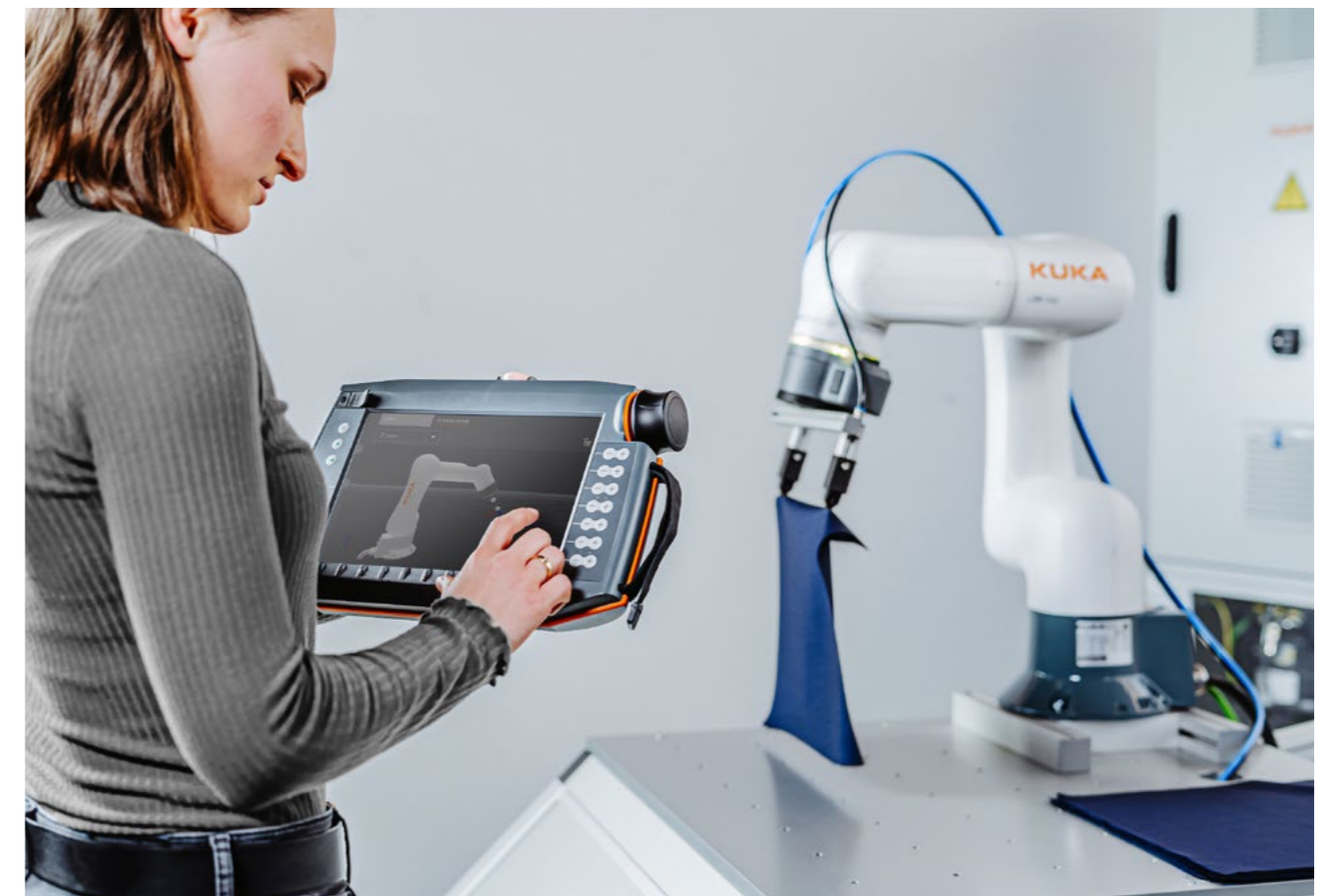
The handling of flexible, easily deformable, flexible textiles and cut parts, is possible with an LBR iisy robot.
