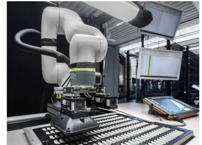
Equipped with cameras, an LBR iisy cobot in conjunction with the iiQKA.OS operating system, checks quality in the plastics industry.
