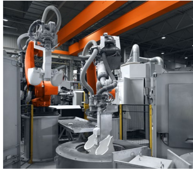
KUKA casting robots for utmost accuracy in ladling, dosing and pouring
