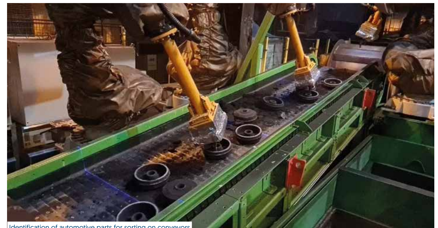
Identification of automotive parts for sorting on conveyors
