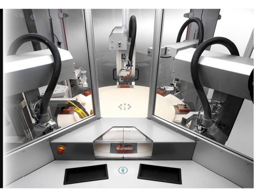
The result of a technological challenge, our Evolubox® cells open a new way in the automated assembly of small and medium series. They allow you to easily automate your industrial production in a progressive way or to share the investment of an automation system over several medium series product lines.
