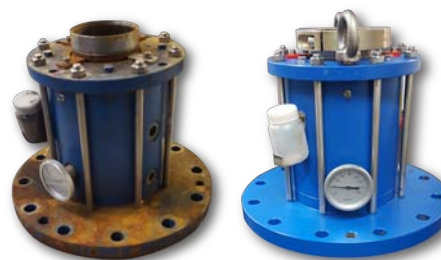
EXAMPLE OF THE RECONDITIONING OF A SEAL CARTRIDGE
