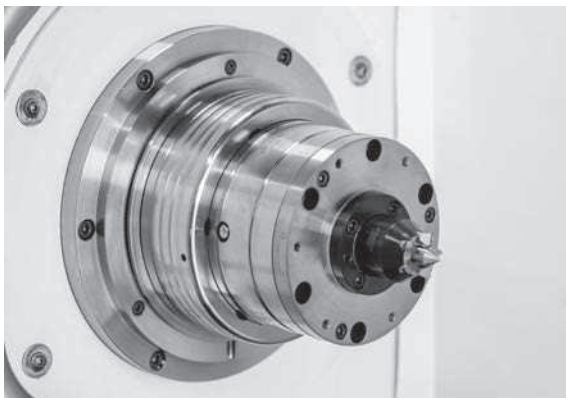
Face driver adaptation on the machine
