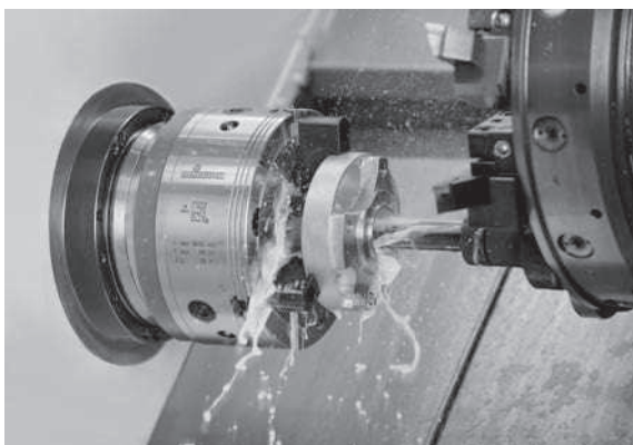
B-Top jaw chuck in use
