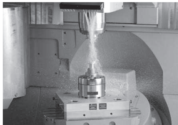
hs dock mandrel actuating unit in use
