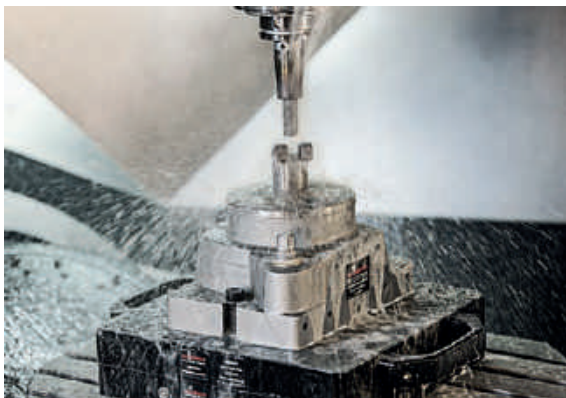
MANOK plus manual stationary chuck in use
