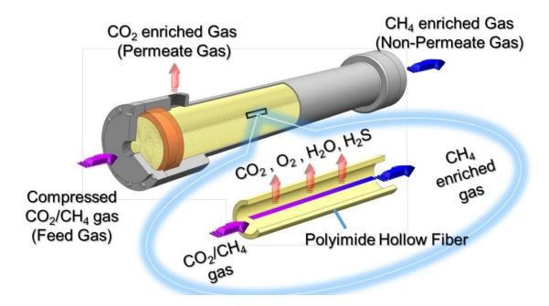
The membranes consist of a bundle of fibres. Each fibre has a diameter of 1 micron or smaller. The  $CO_2$  molecules can be separated fairly easy by the fibres. The  $O_2$ ,  $H_2O$  and  $H_2S$  molecules are more difficult to separate. Luckily are most of the  $H_2O$  and  $H_2S$  molecules already removed before the biogas enters the membranes.
