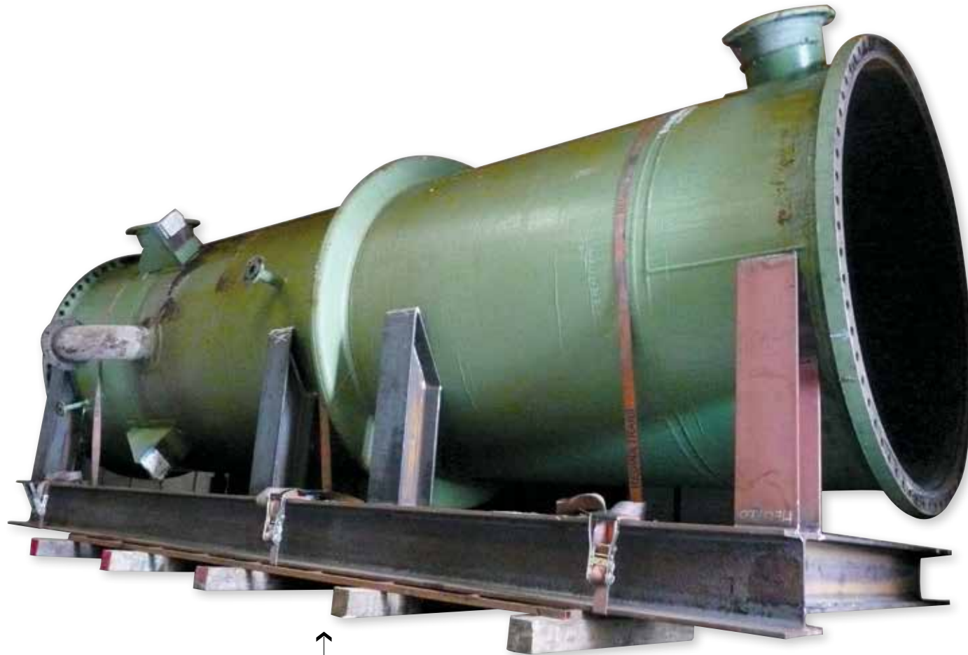
HEAT EXCHANGER WITH COMPENSATOR
