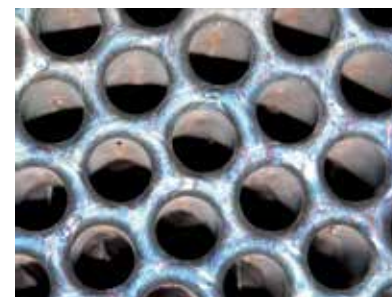
INSIDE TUBES WITH STATIC MIXERS
